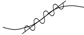
Fig(5). Illustration of the high-frequency approximation. If the wavelength of the wave (wavy line) is much smaller than the distance over which the background space-time varies (curved line), the background can, locally, be taken to be flat (straight line).
