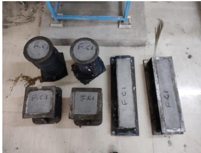
FIG. 7 casting of specimens
